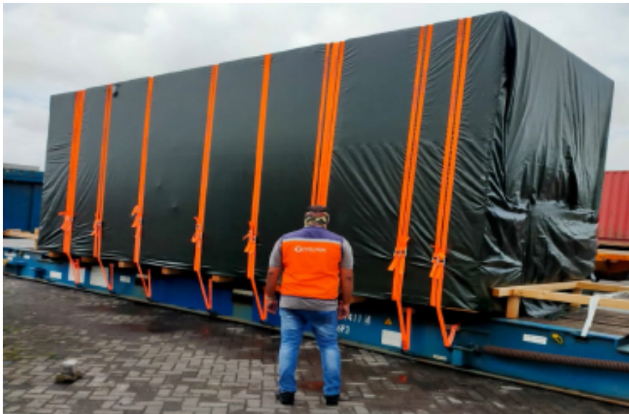
Proper Lashing & choking before exports from India
